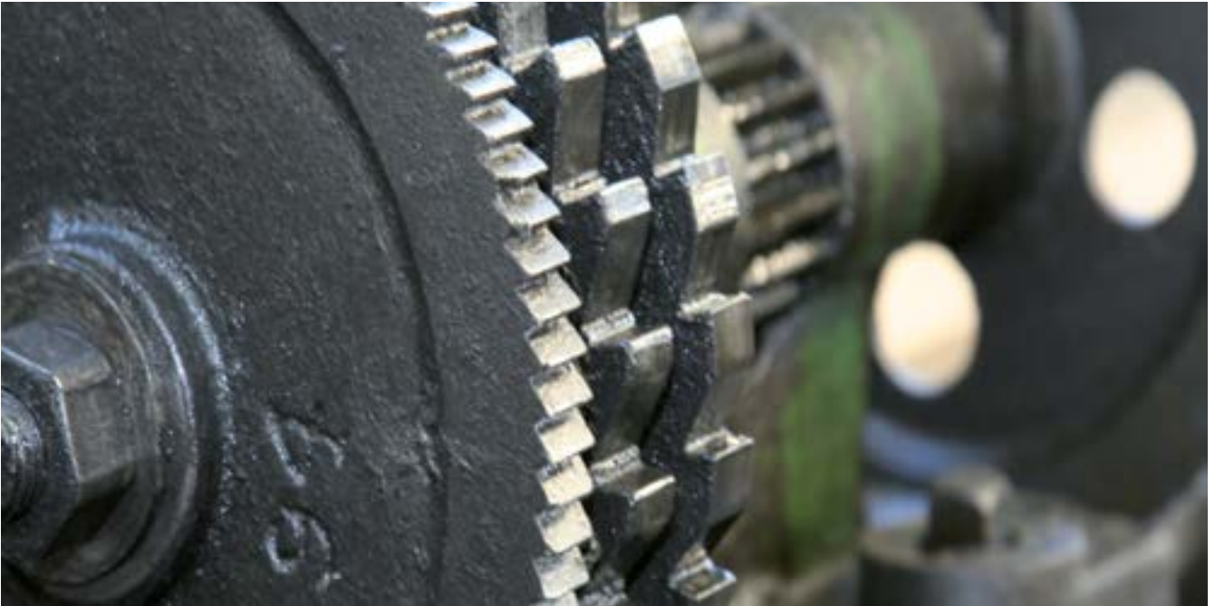
Top: Lock wheel for take-up motion Middle: Division of fabric directly on the bobbinet machine Bottom: Quality control viewing table
